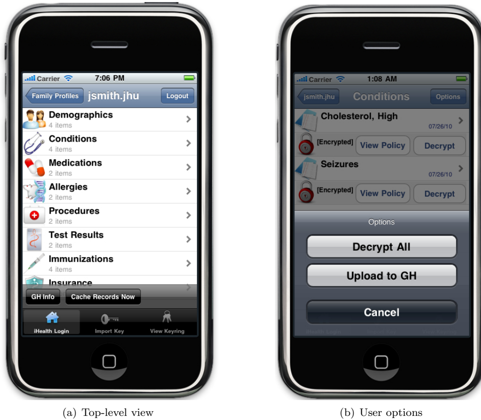
Figure 4: Views of a CCR on our iHealthEMR iPhone application. (a) This view of the application shows the top-level sections of a patient’s CCR. (b) This view of the application shows encrypted entries within a CCR and the access policy the record was encrypted under. Patients may decrypt each individual record or all records within this section as well as upload their records to Google Health.
